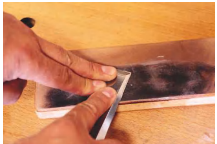
▲ The blackening of strop charged with a honing paste shows that it is removing steel
